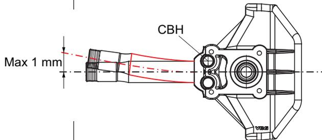
The horizontal bolt must be pressed tightly in and locked using two cylindrical bolts (CBH). The horizontal bolt's thread flanks must not be asymmetrical or damaged; see the picture on the right.
