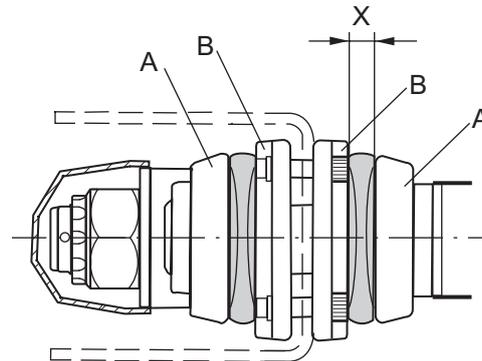
Distance X between the bearing boxes must not exceed X mm when the traction vehicle pushes and pulls heavily (50–80 kN) at the braked trailer.
