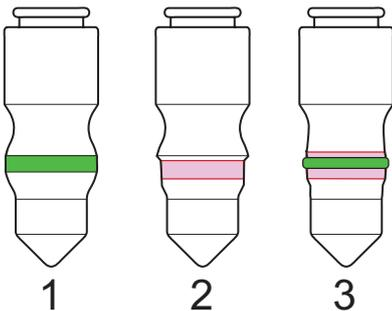
There must be no vertical movement of the coupling bolt when the vehicle is pulling and pushing at the braked trailer. There should be no wear outside of what is indicated in coupling bolt picture 1 or the minimum diameters specified in the table below.
