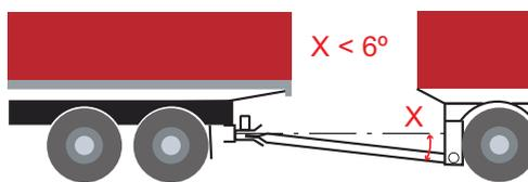
The drawbar closure should be less than 6°.
